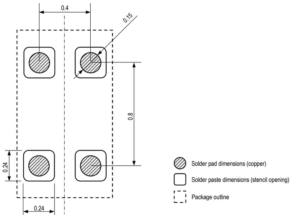
Figure 11 Recommended metal land pattern for SHTW2 (all dimensions are in mm). Recommended solder paste stencil thickness is 75 to 100  $\mu\text{m}$ . The solder pads on the PCB are recommended to be non solder mask defined (NSMD). Copper traces leading towards the solder pads are recommended to have a width of max. 0.09 mm in the direct vicinity of the pads. For general information on land pattern design refer to the IPC-7351 standard.
