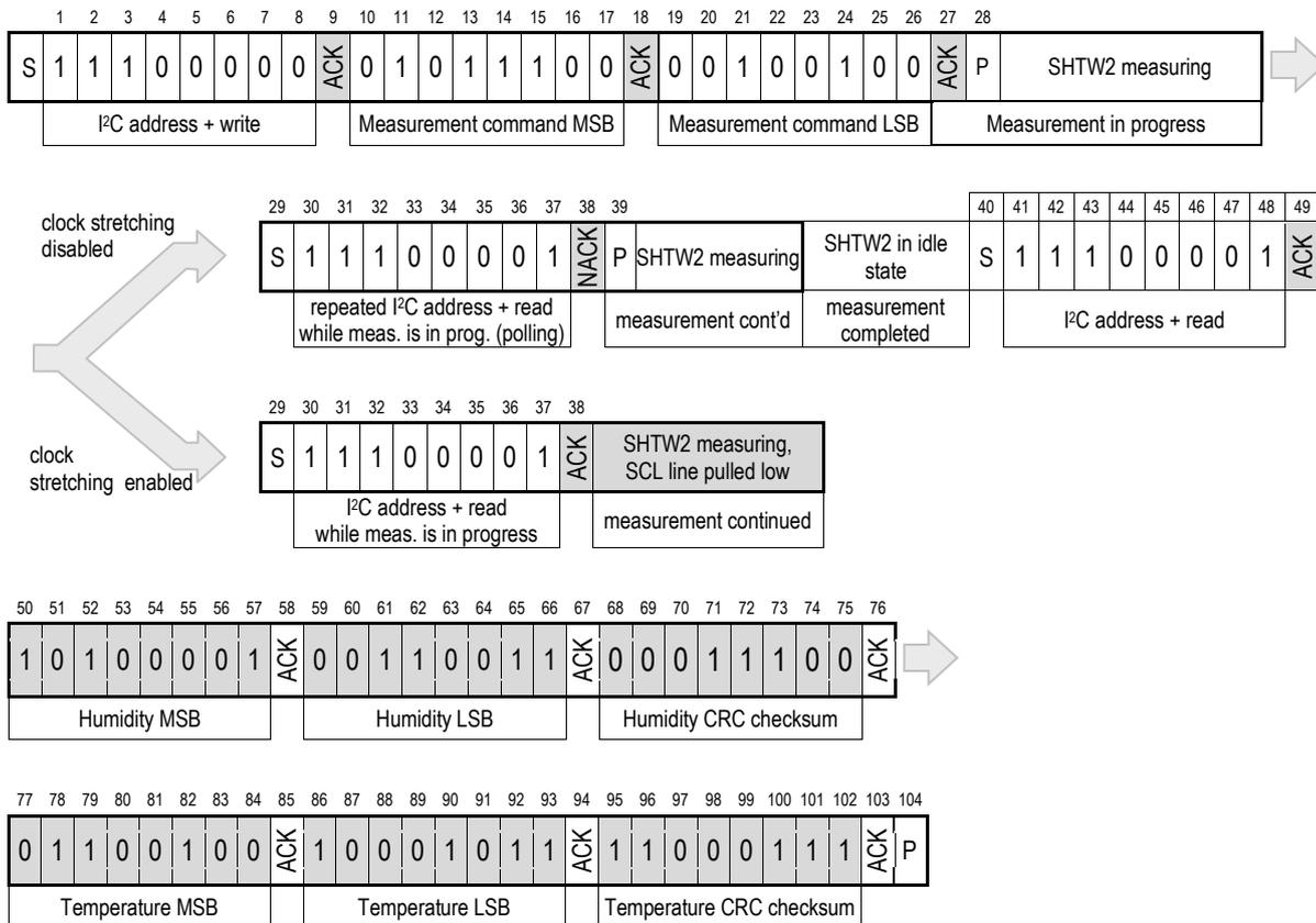
**Figure 7** Communication sequence for starting a measurement and reading measurement results displaying both clock stretching options. The numerical example corresponds to a read humidity-first command with clock stretching enabled. The physical values of the transmitted measurement results are 65.6 %RH and 23.7 °C. Clear blocks are controlled by the microcontroller, grey blocks by the SHTW2.
