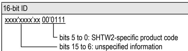
**Table 12** Structure of the 16-bit ID. Bits 15:6 of the ID contain unspecified information (marked as “x”), which may vary from sensor to sensor, while bits 5:0 contain the SHTW2-specific product code.
