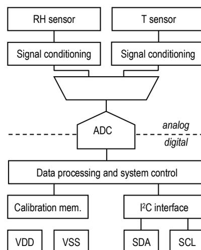
**Figure 1** Functional block diagram of the SHTW2.
