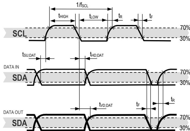
**Figure 5** Timing diagram for digital input/output pads. SDA directions are seen from the sensor. Bold SDA lines are controlled by the sensor, plain SDA lines are controlled by the micro-controller. Note that SDA valid read time is triggered by falling edge of preceding toggle.
