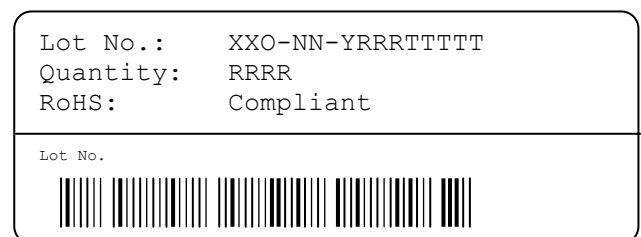
Figure 12: First label on reel: XX = Sensor Type (21 for SHT21), O = Output mode (D = Digital, P = PWM, S = SDM), NN = product revision no., Y = last digit of year, RRR = number of sensors on reel divided by 10 (200 for 2000 units), TTTT = Traceability Code.
