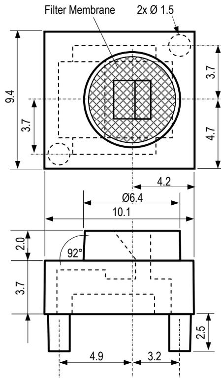
**Figure 1:** Drawing of Filter Cap SF1. Dimensions are given in mm (1mm = 0.039inch), tolerances are  $\pm 0.1$ mm for dimensions  $< 6$ mm and  $\pm 0.2$ mm for dimensions  $> 6$ mm. Cavity inside the cap fits perfectly to SHT1x sensors. Additional cavities for solder joints are left open at each side.
